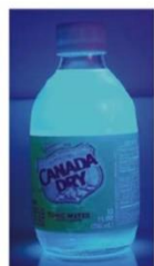
Figure 5.3: Tonic water is clear under normal light, but vividly fluorescent under ultraviolet light, due to the presence of the quinine used as a flavouring.
