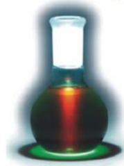
Figure 5.5: A solution of chlorophyll in ether solution shows blood red fluorescence.
